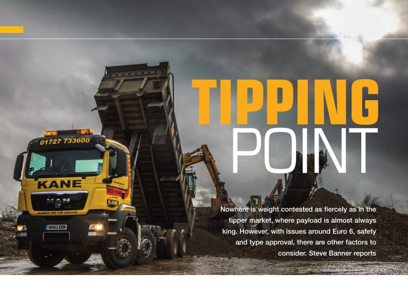
ight-wheeler tippers' permitted gross weights should be increased from 32 to 33 tonnes to compensate for the extra burden imposed by Euro 6 exhaust emission technology and additional safety equipment. So says Trevor Marshall, managing director of tipper builder Aliweld. "For Euro 6, we're looking at up to 300kg extra, depending on the manufacturer," he observes. "And extra safety equipment can mean up to another 200kg."
